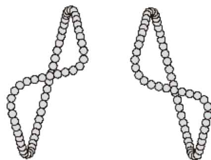
Fig 3.1.4 Internal Ball Circulation Nuts
